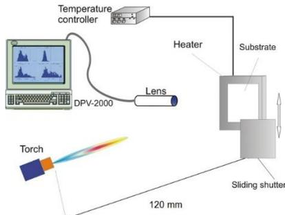
Fig. 2 Schematic of experimental set up
