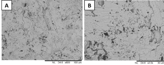
Fig. 8 The microstructure of the splats produced with argon 10% H<sub>2</sub> at different magnifications; A) 800X and B) 2000X
