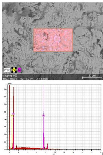
Fig. 5 The EDS spectrum on a single splat produced with no H<sub>2</sub> content gas in the plasma atmosphere mixture showing nickel and oxygen peaks
