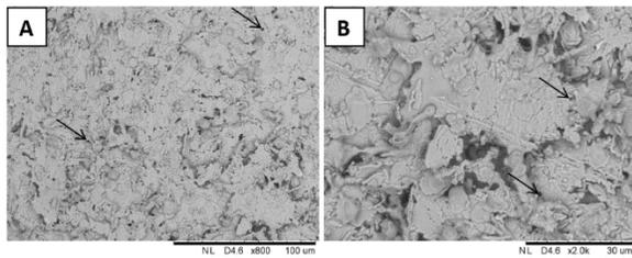
Fig. 4 The microstructure of the splats produced with no H<sub>2</sub> content gas in the plasma atmosphere mixture in different magnifications; A) 800X and B) 2000X
