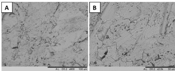
Fig. 9 The microstructure of the splats produced with argon 13% H<sub>2</sub> in the plasma atmosphere mixture in different magnifications; A) 800X and B) 2000X
