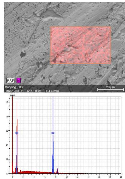
Fig. 7 The EDS spectrum on a single splat produced with 7% H<sub>2</sub> content gas in the plasma atmosphere mixture showing only nickel peaks
