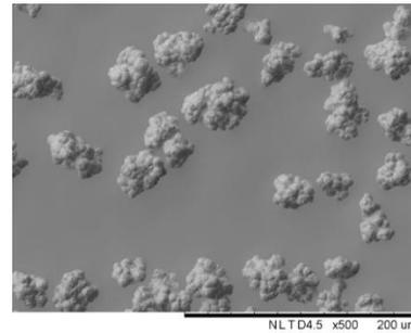
Fig. 3 Nickel powder particles used for plasma spraying
