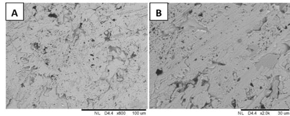
Fig. 6 The microstructure of the splats produced with argon 7% H<sub>2</sub> in the plasma atmosphere mixture in different magnifications; A) 800X and B) 2000X
