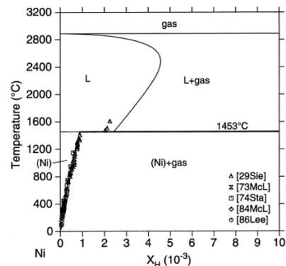
Fig. 1. Ni-rich part of the Ni-H phase diagram, showing hydrogen solubility in liquid and solid states nickel [8]
